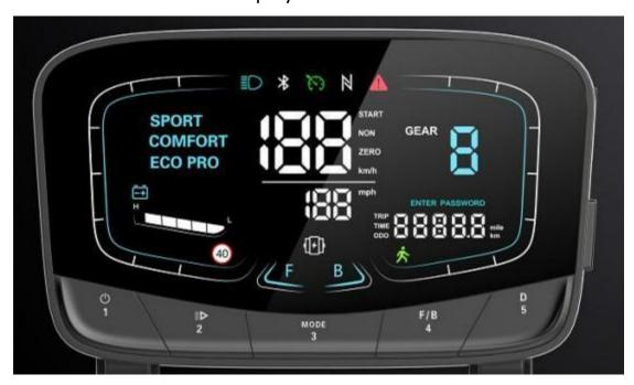
The fault status displays the area E, when the symbol is flashing, press the M/3 key to adjust the display interface to the E interface, the corresponding number under the interface represents the corresponding fault content, the specific status is as follows
